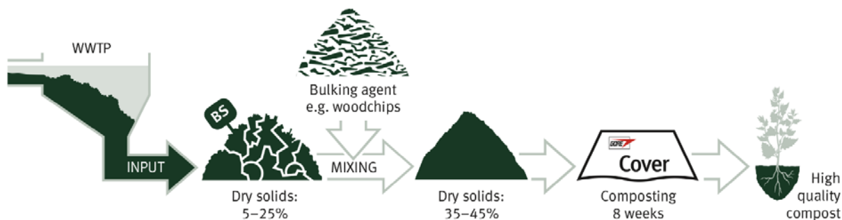
Figure 1. State of the Art technology for organic waste treatment
