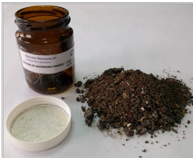
Figure 1. “Sludge incineration ash” resulted from incineration of sewage sludge
