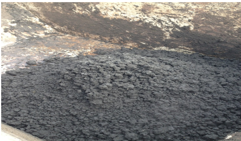
Figure 4. Dehydrated sludge with centrifuge, having 25% solid content
