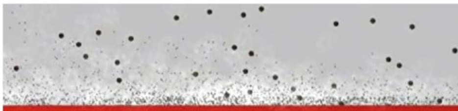
Figure 8. Gravitational separation of dry sludge granules
