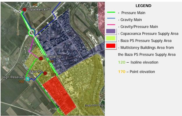
The general scope of project is network optimization through decommissioning of the existing Baza PS and establishment of gravity water supply to the Northern/Central part of Balti from upper reservoirs (190
