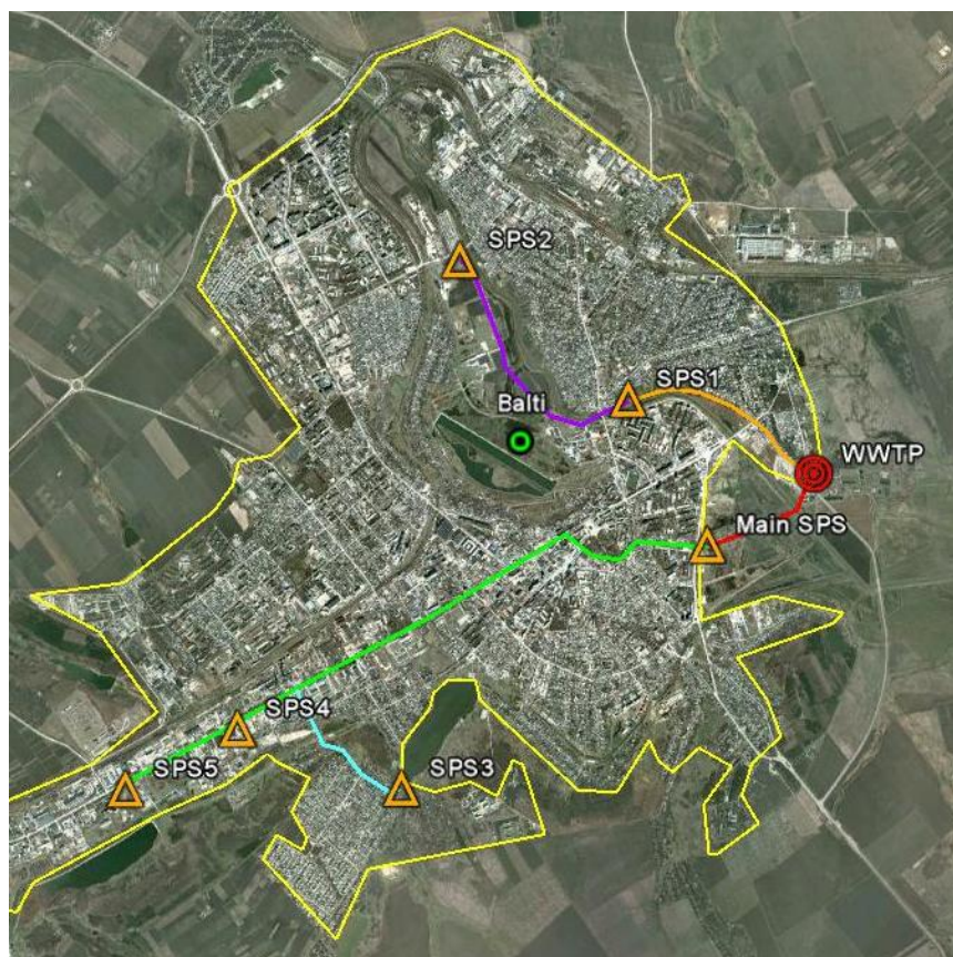
Figure 4-1 Principle Scheme of Sewerage System in Balti
