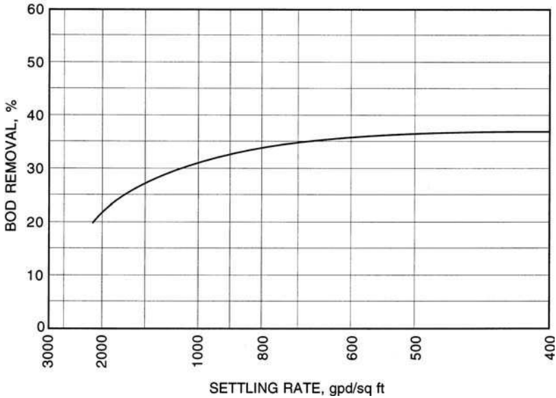
Figure 6.11 BOD 5 removal in primary settling tank (source: Illinois EPA 1998).
