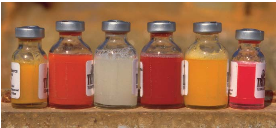
Fig. 79. Selection of microspheres used in the Straßberg/Harz 2003 tracer test.
