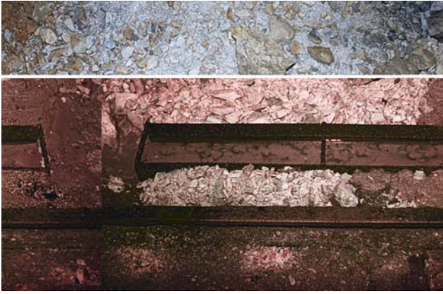
Fig. 50. Badly maintained channel for flow measurements in an underground mine. The channel inflow is not laminar and the channel itself is filled with sediment.
