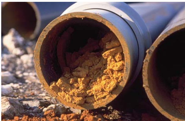
Fig. 8. Ochre precipitates in a mine water discharge pipe of the abandoned Straßberg/Harz fluorspar mine.
