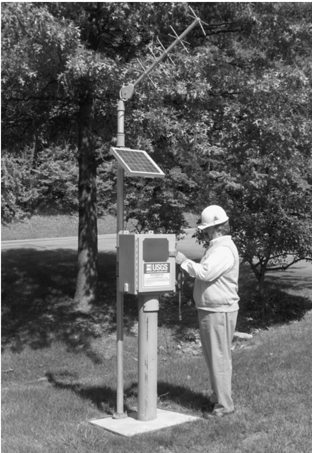
FIGURE 8.13 USGS monitoring well located at the headquarters of the National Ground Water Association in Columbus, OH. Water level data are recorded in real-time and transmitted via satellite to the USGS processing center. The data are available online 15 minutes after recording.
