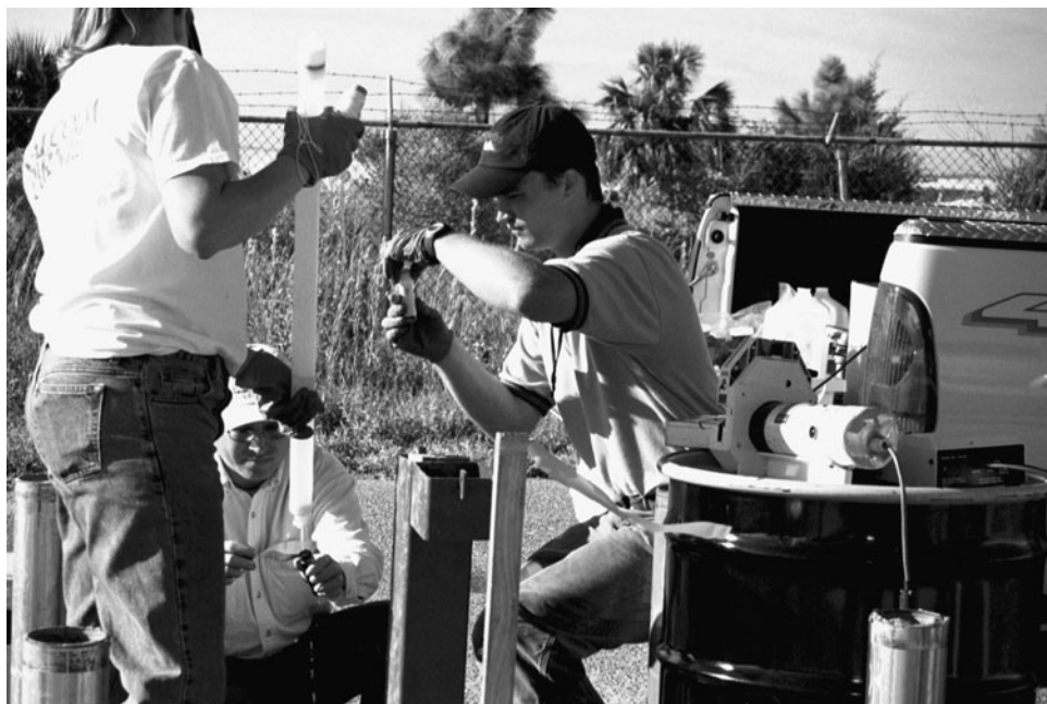
FIGURE 8.19 Collection of groundwater samples at a monitoring well screened in shallow aquifer in the panhandle region of Florida. (Left) Samples are being collected with a Teflon ® bailer.
