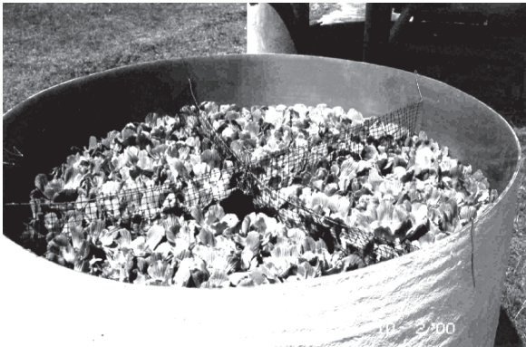
Fig. 24.1 Experimental tank for \mu determination under natural conditions
