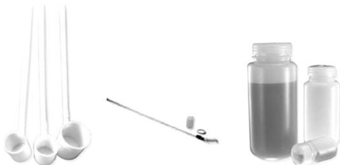
FIGURE 3.4 Various manual sampling devices (from left to right: sample dipper, swing sampler, and sample containers) (USA Bluebook, Waukegan, Illinois).
