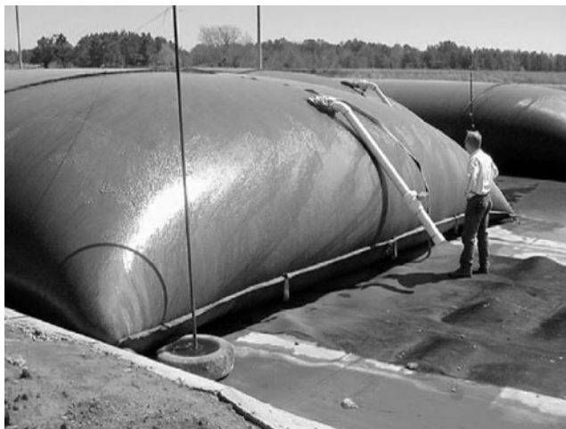
FIGURE 9.26 An example of a typical geotextile system (Geotube ® ) (courtesy of TenCate ™ Geosynthetics North).
