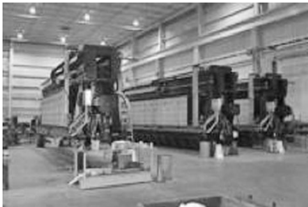
FIGURE 9.22 An example of filter presses at a steel works plant (courtesy of Siemens Water Technologies).
