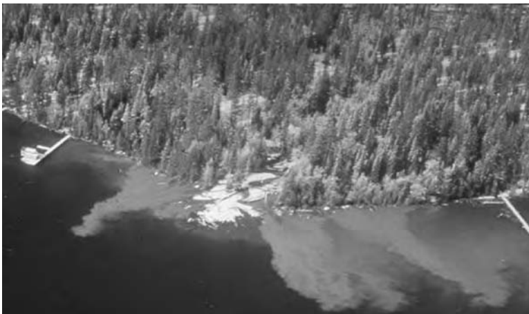
FIGURE 5.15 Nonpoint-source discharge. (From University of Nevada, 2005.)
