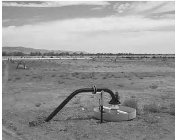
FIGURE 7.7 Injection well. (From Healthgate Resources, 2005.)
