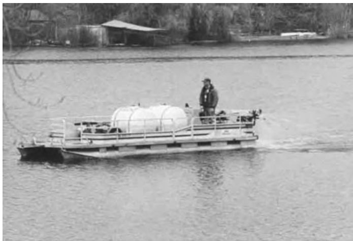
FIGURE 5.16 Alum treatment. (From Allied Biological, 2005.)
