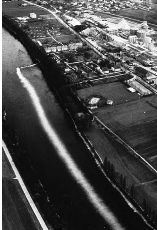
FIGURE 4.1 Contaminant discharge into the Alpenrhein River, Germany. (From Socolofsky and Jirka, 2005.)
