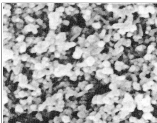
(x 10,000, electron microscopic photograph) Photo 2.21 Particles of iron oxide (without polymer dispersant)
