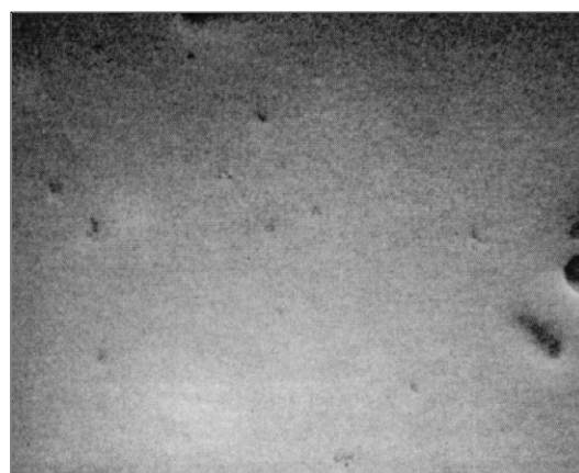
(Secondary electron image x 10,000) Photo 2.25 Particles of magnetite dispersed by polymer I treatment
