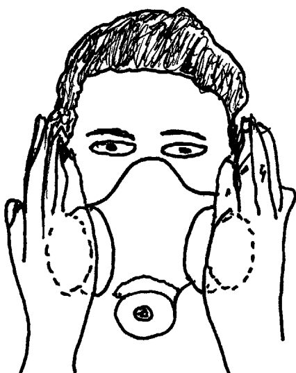
FIGURE 3.12. Fit test—self-test—negative pressure.
