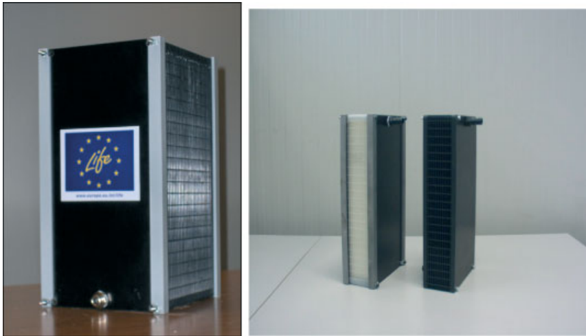
Figure 22.3 Picture of two membrane contactors each housing 1 m 2 of membrane (right) and 1 contactor housing 3 m 2 of membrane (left).
