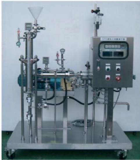
Figure 21.12 Marketed equipments for membrane emulsification. (a) Plant for crossflow membrane emulsification produced by SPG Technologies Co. Ltd ( http://www.spg-techno.co.jp/ ); (b) spiral-wound metallic membrane module produced by Micropore Technologies ( http://www.micropore.co.uk/ ).
