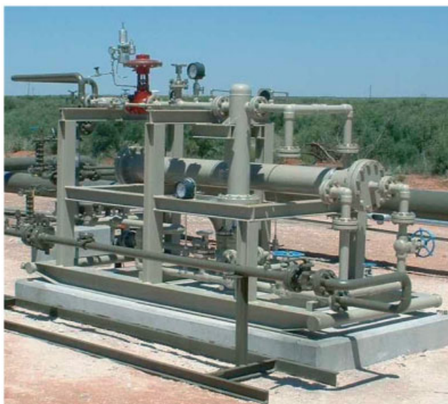
Figure 8.12 Block diagram and photograph of a membrane fuel-gas conditioning unit (FGCU) used for a field gas compressor engine (the unit uses silicone rubber membranes in spiral-wound modules). The membrane modules are
