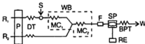
Fig. 2.31 Schematic flow diagram for the determination of nitrite R_1 , p -aminoacetophenone solution (5g plus 10ml conc. hydrochloric acid diluted to 500ml diluted to 40ml to 1L); R_2 , m -phenylenediamine solution (13.8g m -phenylene dihydrochloride, diluted in 500ml water, diluted 40ml to 1L); P, double plunger micro pump ( 1.7\text{ml min}^{-1} ); DT, damping coil ( 0.5\text{mm id}\times 20\text{m} ); S, loop valve sample injector (sample volume 650\mu\text{L} ); WB, water bath 30^\circ\text{C} ; MC 1, mixing coil ( 1\text{mm id}\times 150\text{cm} ); MC 2, mixing coil ( 1\text{mm id}\times 100\text{cm} ); F, line filter; SP, spectrophotometer with flow cell (light path 10mm, 8\mu\text{L} ); RE, recorder, BPT, back pressure coil ( 0.5\text{mm id}\times 5\text{m} ); W, water
