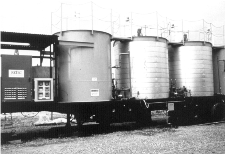
Large-scale complete mix pilot reactors are used to evaluate bioslurry treatment technologies. Courtesy of Remediation Technologies, Inc.
