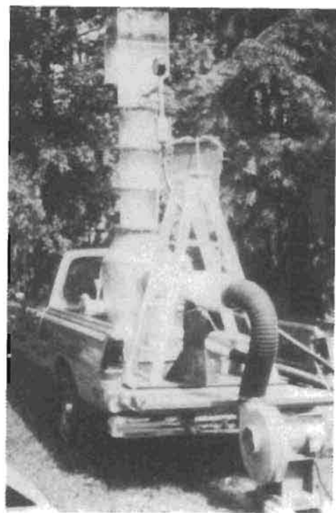
Pilot catenary grid aerator unit.
