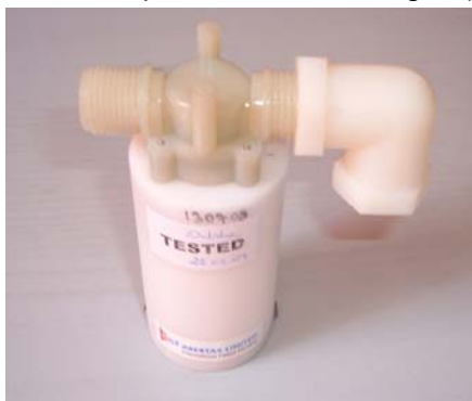
Figure 6: Two Solutions to Meter Under-Registration: The Magnetic Water Inlet Valve (Left) and the Unmeasured Flow Reducer (Right)
