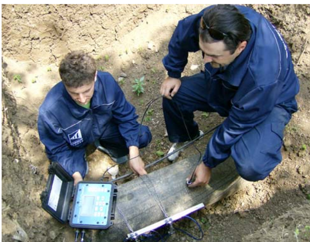
Figure 4. Flow measuring with Ultrasonic mobile flow meter
