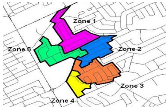
Figure 16: Zones used for flow step testing in the cast iron pipe DMA in Meadowlands
