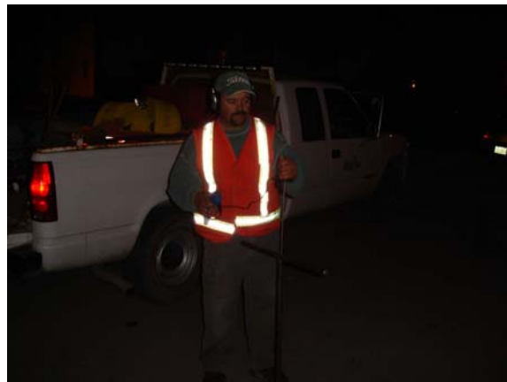
Figure 4: Acoustic listening to check boundary valves
